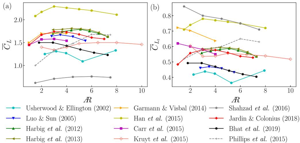
**FIG. 11.** Comparison of variations in (a) the lift coefficient based on  $U_g$  ( $\bar{C}_L$ ) with  $\mathcal{AR}$  and of those in (b) the lift coefficient based on  $U_t$  ( $\bar{C}_{L_t}$ ) with  $\mathcal{AR}$ , extracted from various past studies, is shown. The dashed line represents the LEV-circulatory lift coefficient.
