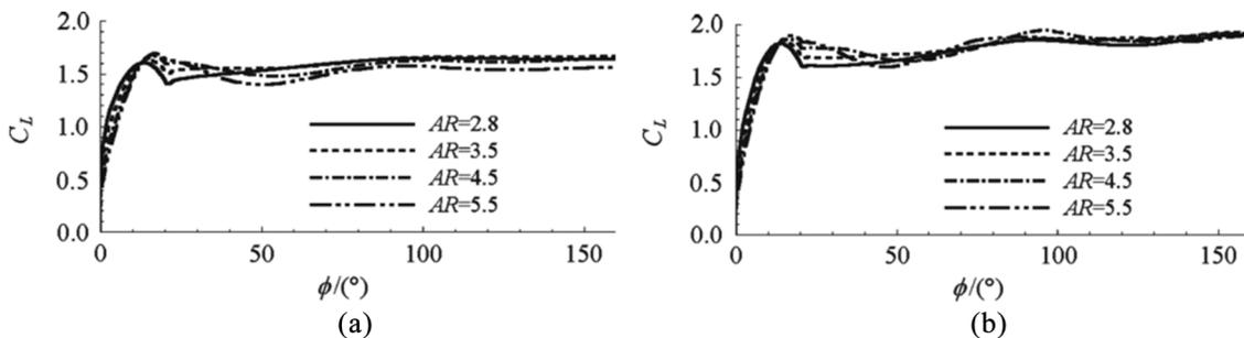
FIG. 9. Variation of  $C_L$  with the sweep angle  $\phi$  shows a negligible effect of  $\mathcal{AR}$  at (a)  $Re = 200$  and (b)  $Re = 3500$ . Figure adapted with permission from G. Luo and M. Sun, "The effects of corrugation and wing planform on the aerodynamic force production of sweeping model insect wings," *Acta Mech. Sin.* **21**, 531–541 (2005). Copyright 2005 Springer Nature.
