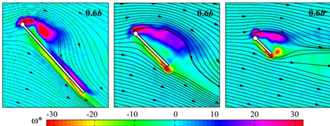
**FIG. 6.** The contours of the normalized vorticity ( $\omega^* = \omega \bar{c} / U_i$ ) are superimposed with the streamlines of flow over wings of  $\mathcal{AR} = 1.5, 3,$  and  $6$  at  $r/b = 0.6$ . Figure adapted with permission from J.-S. Han, J. W. Chang, and H.-K. Cho, "Vortices behavior depending on the aspect ratio of an insect-like flapping wing in hover," *Exp. Fluids* **56**, 181 (2015). Copyright 2015 Springer Nature.
