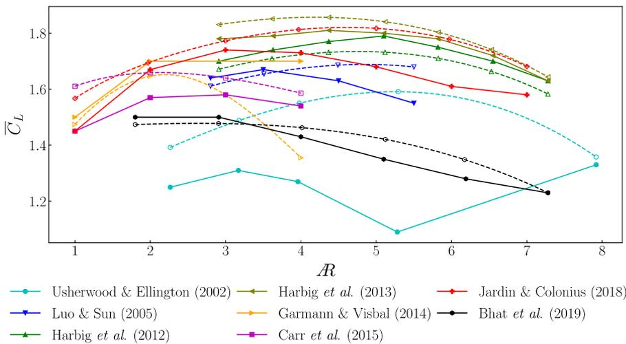
**FIG. 16.** The variations in  $\bar{C}_L$  reported by previous researchers are compared with the predictions using the polynomial model, shown by open symbols and dashed lines of the corresponding colors.
