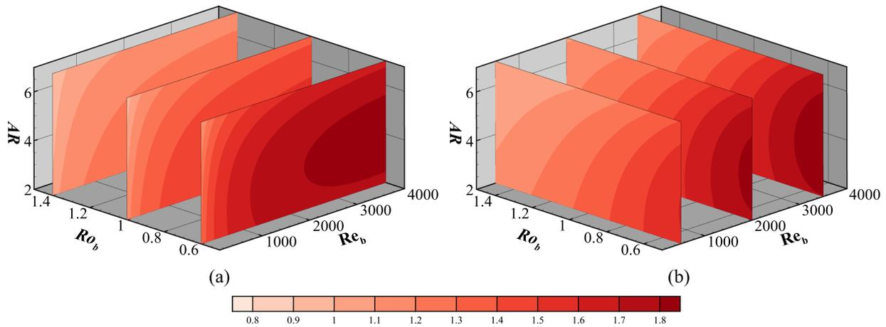
**FIG. 15.** The contours of  $\bar{C}_L$ , predicted using the polynomial model, are shown in the 3D space of  $\mathcal{AR}$ ,  $Re_b$ , and  $Ro_b$  in (a) on the  $\mathcal{AR} - Re_b$  planes at  $Ro_b = 0.6, 1, \text{ and } 1.4$  and in (b) on the  $\mathcal{AR} - Ro_b$  planes at  $Re_b = 500, 2000, \text{ and } 3500$ .
