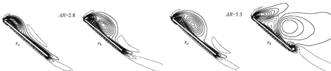
**FIG. 5.** Vorticity contours over a wing are shown at two different spanwise locations for  $\mathcal{AR} = 2.8$  and  $\mathcal{AR} = 5.5$ .  $r_a$  and  $r_b$  represent the locations  $r/b = 0.4$  and  $r/b = 0.6$ , respectively. Figure adapted with permission from G. Luo and M. Sun, “The effects of corrugation and wing planform on the aerodynamic force production of sweeping model insect wings,” *Acta Mech. Sin.* **21**, 531–541 (2005). Copyright 2005 Springer Nature.
