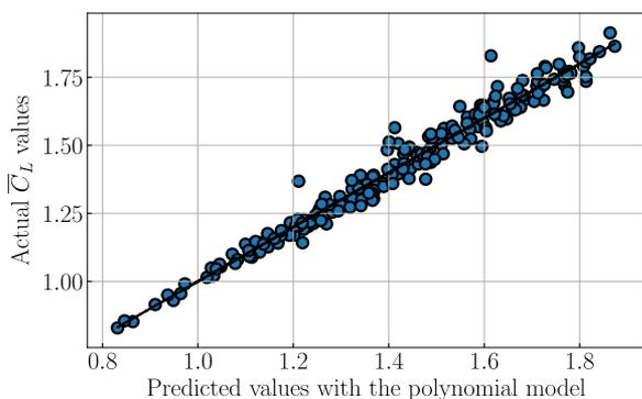
**FIG. 17.** The comparison of the actual  $\bar{C}_L$  values and the predicted values using the polynomial model.
