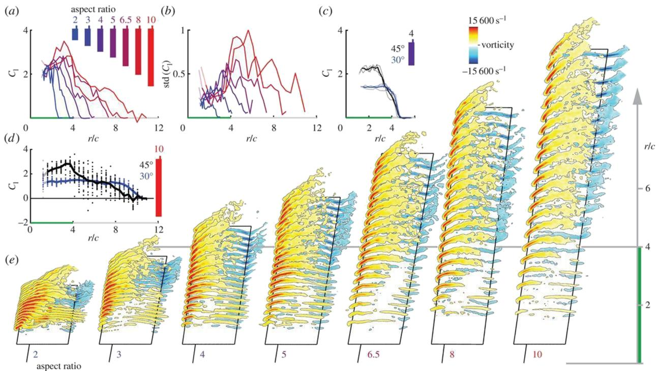
**FIG. 4.** The vorticity contours inside the LEV core at various spanwise sections are shown for various  $\mathcal{AR}$ . Republished with permission from Kruyt *et al.*, “Power reduction and the radial limit of stall delay in revolving wings of different aspect ratio,” *J. R. Soc., Interface* **12**, 20150051 (2015). Copyright 2015 Royal Society.
