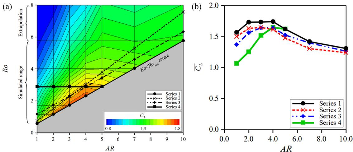
**FIG. 13.** In (a), contours of  $\bar{C}_L$  are mapped on the plane of  $\mathcal{R}$  and  $Ro$ . In (b), the variations in  $\bar{C}_L$  with  $\mathcal{R}$  are shown for various series of configurations. Figures adapted with permission from Y. J. Lee, K. B. Lua, and T. T. Lim, “Aspect ratio effects on revolving wings with Rossby number consideration,” *Bioinspiration Biomimetics* 11, 056013 (2016). Copyright 2016 IOP Publishing.
