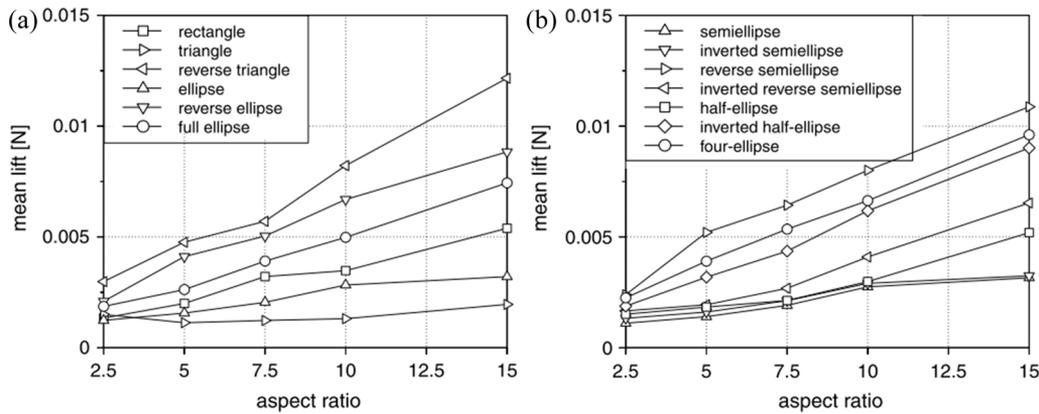
FIG. 8. Relation between lift and  $\mathcal{AR}$  for (a) symmetric and (b) asymmetric wing shapes is shown. Figure reproduced with permission from S. A. Ansari, K. Knowles, and R. Zbikowski, "Insectlike flapping wings in the hover. Part I: Effect of wing kinematics," *J. Aircr.* **45**, 1945–1954 (2008). Copyright 2008 by S. A. Ansari.
