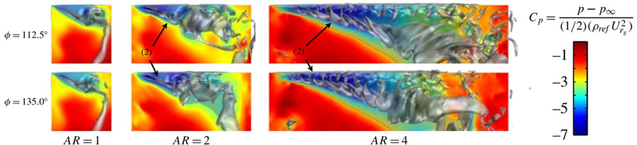
**FIG. 7.** The 3D LEV structure, identified using the isosurface of total pressure, changes significantly with  $\mathcal{AR}$ . Contours of the pressure coefficient are shown on the wing suction surface. Figure adapted with permission from D. J. Garmann and M. R. Visbal, "Dynamics of revolving wings for various aspect ratios," *J. Fluid Mech.* **748**, 932–956 (2014). Copyright 2014 Cambridge University Press.
