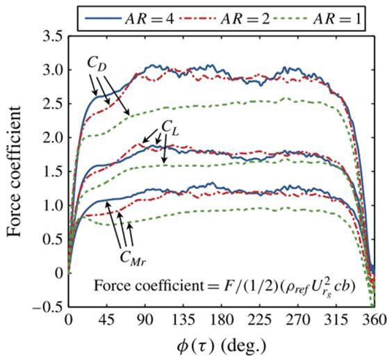
**FIG. 10.** Variations in force coefficients with the sweep angle are shown for various  $\mathcal{AR}$ . Figure adapted with permission from D. J. Garmann and M. R. Visbal, “Dynamics of revolving wings for various aspect ratios,” *J. Fluid Mech.* **748**, 932–956 (2014). Copyright 2014 Cambridge University Press.
