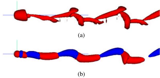
Figure 2: Flow past single sphere,  $Re = 300$ . (a) Iso-surface plot of the vortical wake flow identified by eigenvalue method: side view. (b) Axial vorticity,  $\omega_x$ : top view. Dark:  $\omega = +0.1U/d$ , Light:  $\omega = -0.1U/d$ .
