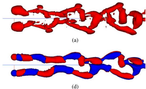
Figure 6: Flow past two spheres,  $S/d = 2.5$ ,  $Re = 300$ . Top view. Contour levels same as Figure 2. (a) Vortical structure in the wake, (b) Axial vorticity,  $\omega_x$ .
