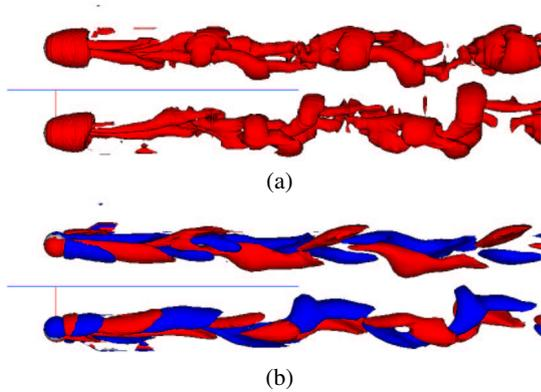
Figure 4: Flow past two spheres,  $S/d = 3.5$ ,  $Re = 300$ . Top view. Contour levels same as Figure 2. (a) Vortical structure in the wake. (b) Axial vorticity,  $\omega_x$ .
