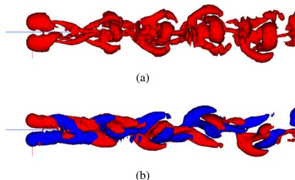
Figure 8: Flow past two spheres,  $S/d = 1.5$ ,  $Re = 300$ . Contour levels same as Figure 2. (a) Vortical wake structure. Top view. (b) Axial vorticity,  $\omega_x$ . Top view.
