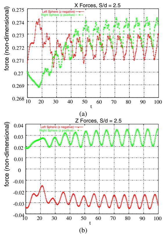
Figure 5: Forces on a two spheres at  $Re = 300$ ,  $S/d = 2.5$ . (a) Axial non-dimensional force. (b) Sideways forces on spheres.
