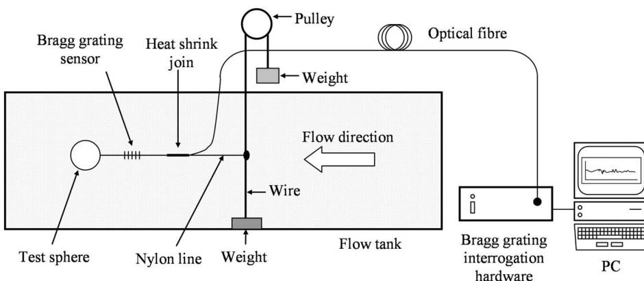
FIG. 1. Flow tank arrangement used to test the drag force on neutrally buoyant spheres.
