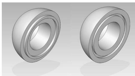
FIG. 3. Modified design of neutrally buoyant spheres, showing the two-halves which connect together.
