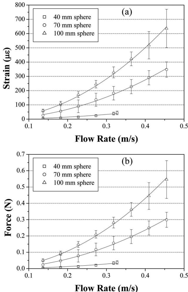
FIG. 6. (a) Strain and (b) drag force vs flow rate for the various spheres tested.
