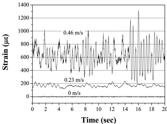
FIG. 5. As for Fig. 4(a) but with reduced time range to show vortex-induced vibrations at increased flow rates.
