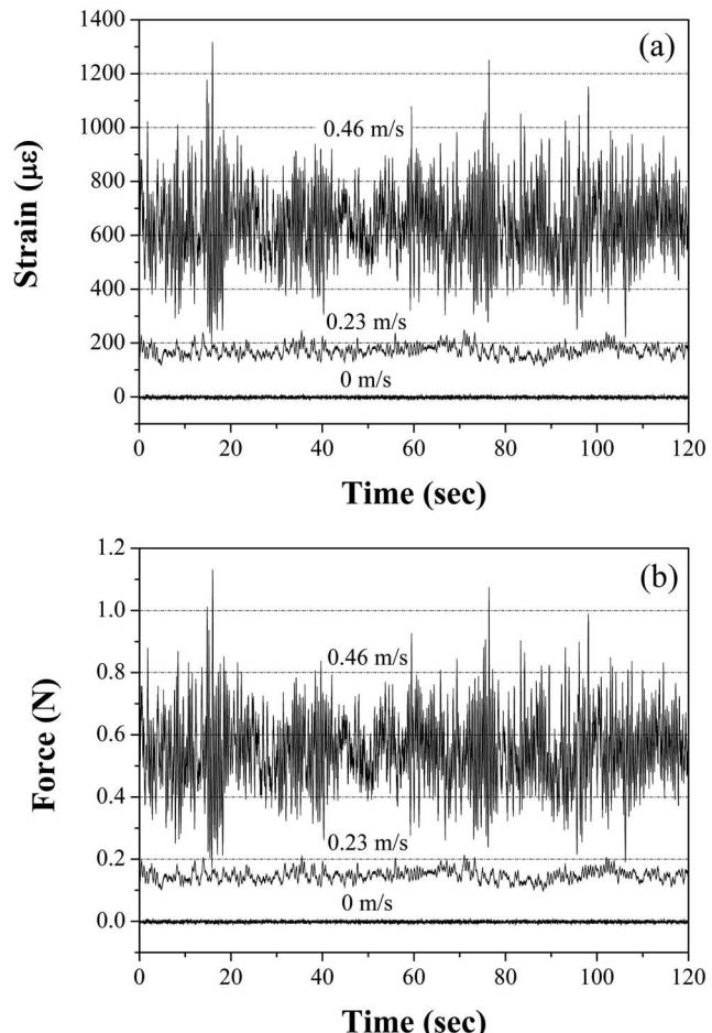
FIG. 4. (a) Strain and (b) drag force on 100 mm diameter sphere in flow tank vs time at various flow rates (tether length of 1 m).
