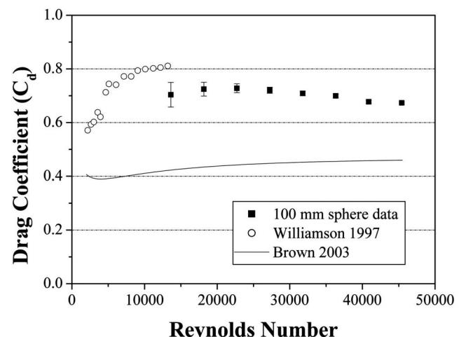
FIG. 7. Comparison of the sphere drag coefficient data obtained for the 100 mm sphere in this work with the values obtained by others.
