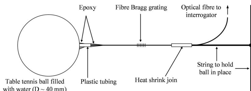
FIG. 2. Detail of the initial sensing and tether arrangement (Note: not to scale).
