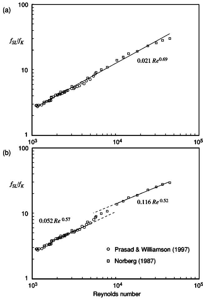
FIG. 1. (a) Variation of the shear-layer frequency ratio with Reynolds number from the studies of Prasad and Williamson (Ref. 4) and Norberg (Ref. 7). The line of best fit to the data is shown. (b) Proposed alternative fit to the data.
