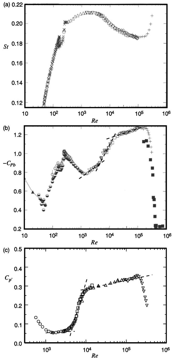
FIG. 2. (a) Strouhal number, (b) base suction coefficient, and (c) fluctuating lift coefficient at  $90^\circ$ , as functions of Reynolds number. These plots have been reconstructed from Fig. 3 of Norberg (Refs. 7 and 8) and Fig. 6 of Norberg (Ref. 9). The overlaid dashed line segment appearing in the last plot highlights the relatively constant behavior within ranges 1 and 2.
