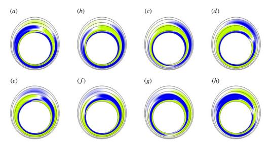
FIGURE 6. (Colour online) Spanwise perturbation vorticity contours of the mode F' instability over one period of shedding at  $\alpha = 6$ , Re = 320 and  $\lambda/D = 0.3$ , with streamlines in the vicinity of the cylinder overlaid: (a) T = 0, T; (b) T = T/8; (c) T = 2T/8; (d) T = 3T/8; (e) T = 4T/8; (f) T = 5T/8; (g) T = 6T/8; (h) T = 7T/8.
