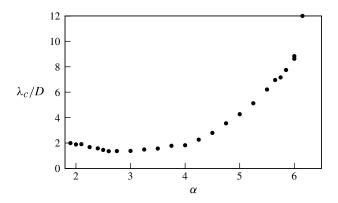
FIGURE 4. Variation of the critical spanwise wavelength with rotation rate for the mode E instability. The wavelength begins to increase exponentially around  $\alpha = 2.5$ , close to where the recirculation region in the wake disappears.
