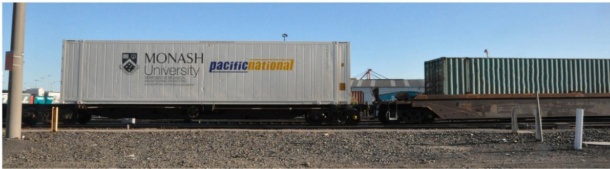
Fig. 1. Instrumented 48-foot (14.6 m) refrigeration shipping container (white) on-board an operational freight train with significantly flatter external ridges than conventional containers (green). (For interpretation of the references to colour in this figure legend, the reader is referred to the web version of this article.)
