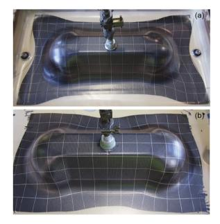
Fig. 11. Formed double dome samples for: (a)  $90^{\circ}/0^{\circ}$  and, (b)  $-45^{\circ}/45^{\circ}$  cases.
