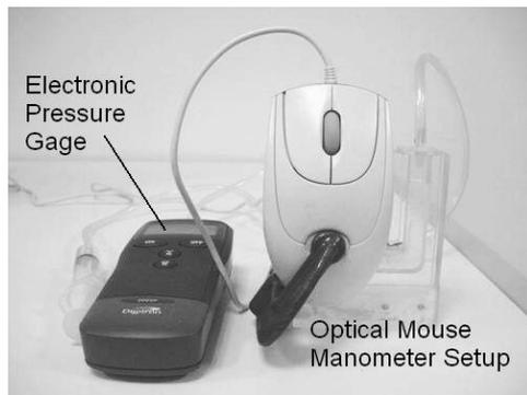
**Figure 3.** Pictorial description of simultaneous pressure measurement with the optical mouse manometer setup, and electronic pressure gauge.
