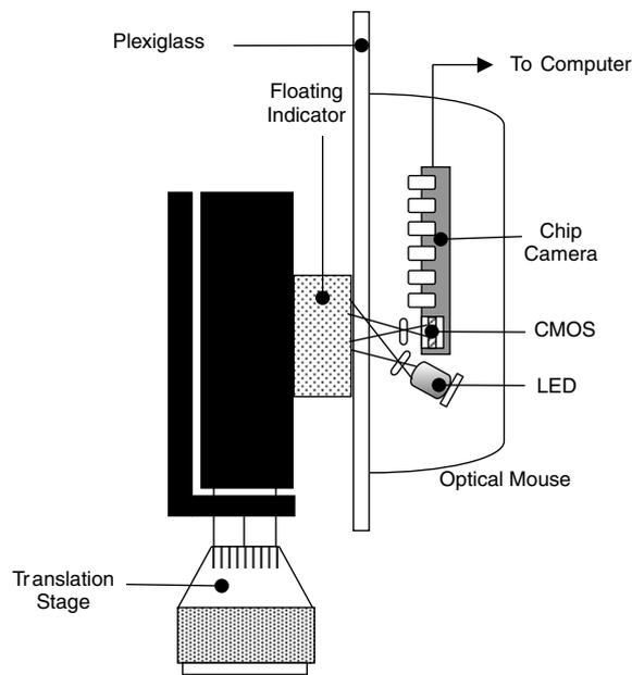
**Figure 2.** Schematic description of the setup to calibrate the translation sensitivity of the optical mouse.
