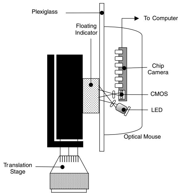
**Figure 2.** Schematic description of the setup to calibrate the translation sensitivity of the optical mouse.
