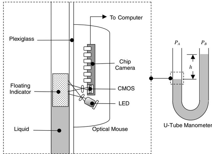
**Figure 1.** Schematic description of the setup to obtain digital readouts for automated data acquisition from a simple U-tube manometer using an optical mouse.
