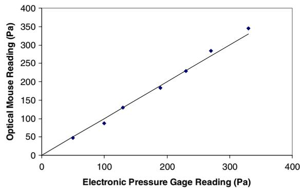
**Figure 5.** Typical plot of pressure determined using the optical mouse incorporated with a U-tube manometer against pressure determined using an electronic pressure gauge. The solid line indicates perfect correlation.
