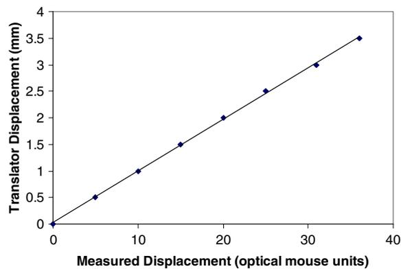
**Figure 4.** Calibrated plot of translator displacement against optical mouse displacement sensing units. The solid line indicates a best fit of the data points.
