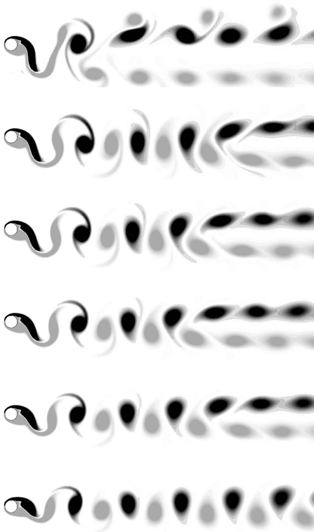
FIG. 7. Variation of the wake with increasing amplitude. Re=200 , f/f_{St}=1.01 , 0.2 \leq A^* \leq 0.7 , increasing in steps of \Delta A^*=0.1 . A^* increases up the page. C_E=0 is traversed at A^* \approx 0.52 , yet the wake is very similar at A^*=0.5 and A^*=0.6 .
