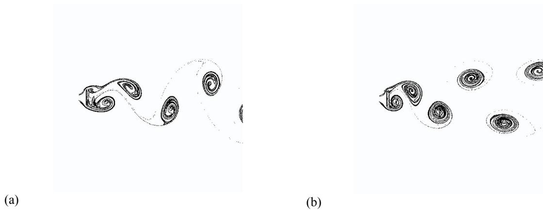
**Figure 5.** Two-dimensional particle traces showing the shedding pattern for flow past a normal flat plate. Flow is from left to right. (a)  $Re = 40$ ; (b)  $Re = 100$ .
