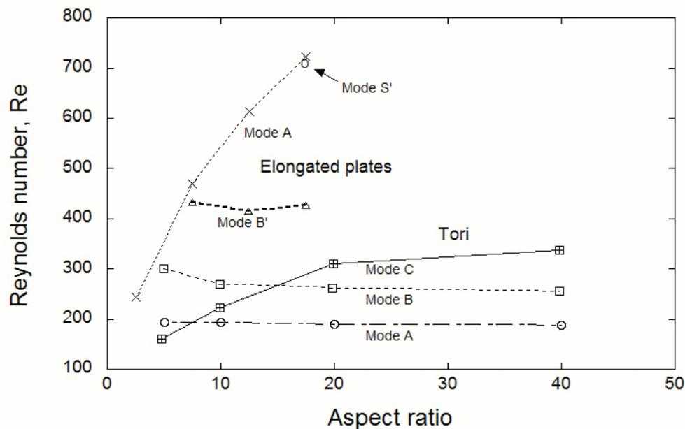
**Figure 8.** Critical Reynolds number for the onset of modes A, B and C for tori for aspect ratios  $AR > 5$ , and for modes A, B' and S' for elongated plates.
