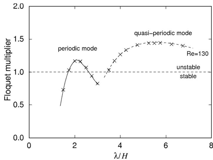
**Figure 6.** Dominant Floquet multipliers for the wake of a normal flat plate.  $Re = 130$ .
