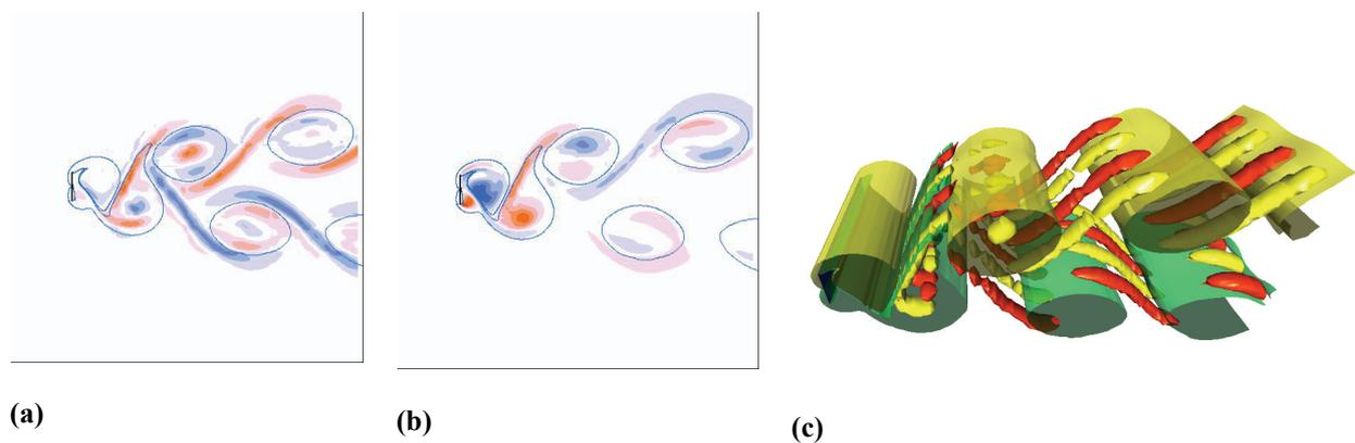
**Figure 7.** Streamwise perturbation vorticity structure of the first two instability modes for the normal flat plate,  $Re = 130$ , for wavelengths of (a)  $\lambda/H = 2.25$  and (b)  $\lambda/H = 5.25$ , respectively. (c) 3d image of the periodic mode -  $\lambda/H = 2.25$ , showing positions of 2d vortices and the streamwise perturbation vortices.  $H$  is the plate height, flow from left to right.
