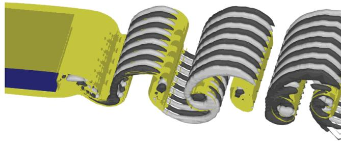
**Figure 10.** Stream-wise and span-wise vorticity components for mode S' in the wake of an elongated cylinder with AR = 12.5.
