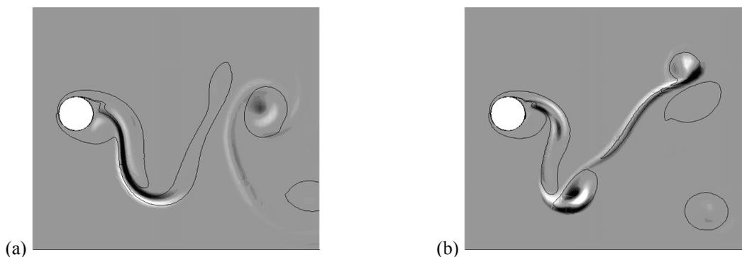
**Figure 11.** Spanwise perturbation vorticity for (a) mode SL,  $A^* = 0.7$ ,  $Re = 200$  and  $\lambda = 1.5$  and (b) mode SS,  $A^* = 0.75$ ,  $Re = 265$  and  $\lambda = 0.80$ , of a transversely oscillating cylinder.
