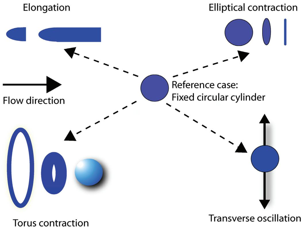
**Figure 3** Four variations on the fixed circular cylinder case considered.
