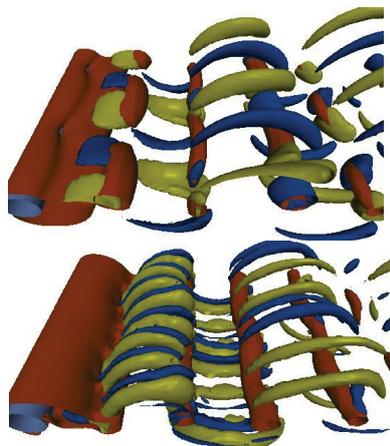
**Figure 1.** Numerical visualisations of the wake streamwise vorticity for the two shedding modes for a fixed circular cylinder. Mode A ( $Re = 210$ ) is at top and Mode B ( $Re = 250$ ) is on bottom.
