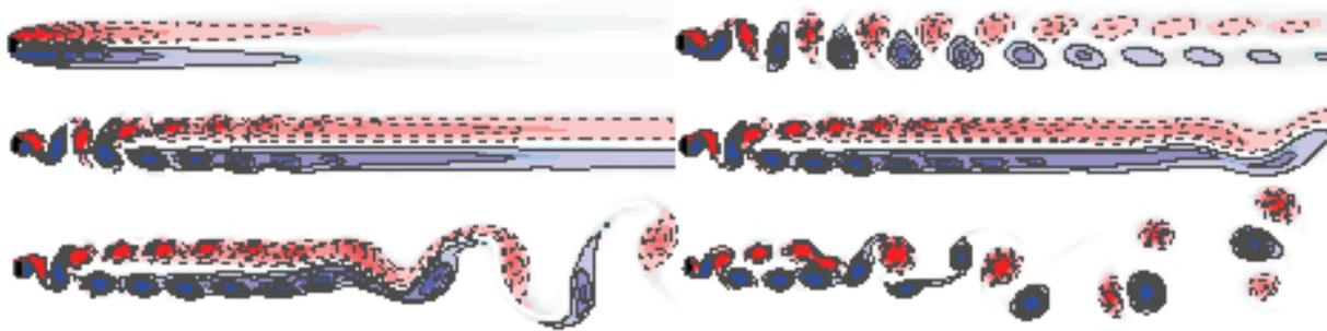
**Figure 4.** Instantaneous vorticity and streamlines showing wake development for AR=0.5 and Re = 40, 75, 125, 150, 175 and 250 (from left to right, then down). Flow from left to right.
