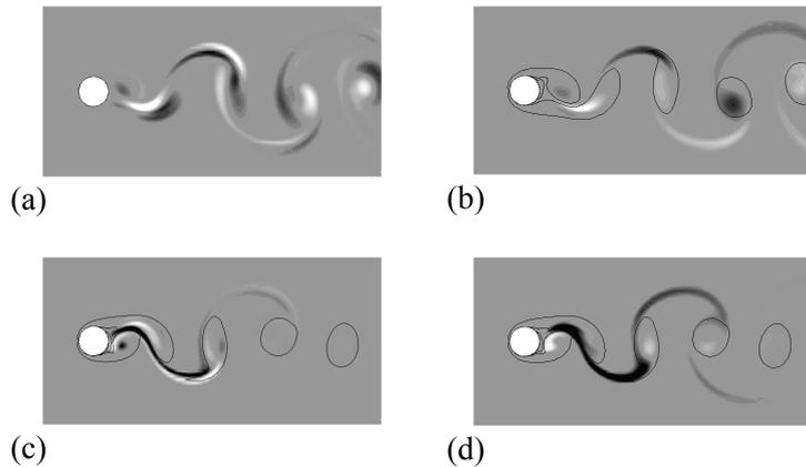
**Figure 2.** (a) Linear perturbation spanwise and (b) streamwise vorticity for mode A in the wake of a fixed cylinder,  $Re = 190$ ,  $\lambda = 3.0$ . The mode has just become unstable. (c) Linear perturbation spanwise and (d) streamwise vorticity for mode B in the wake of a fixed cylinder,  $Re = 260$ ,  $\lambda = 0.75$ . Again, the mode has just become unstable.
