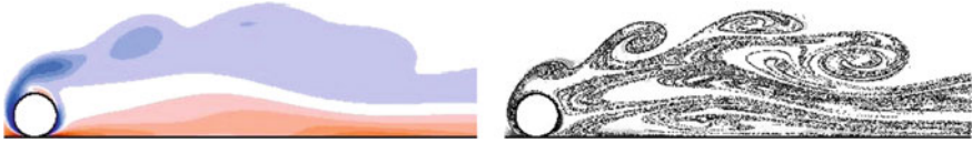
Fig. 7 Numerical flow visualisation of the shear-layer vortices in the wake of the cylinder at Re = 88 , \theta = 1.9^\circ , \beta = 1.10 and r = 2\% . The image on the left shows vorticity contours and the one on the right shows a visualisation of the wake using passive tracer particles released near the rear surface of the cylinder
