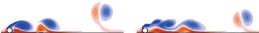
Fig. 6 Coloured vorticity contour showing the effect of an offset centre-of-mass on the wake flow. Left Unperturbed flow. Right Perturbed flow for r = 3\% . Re = 115 , \beta = 1.10 and \theta = 1.9^\circ
