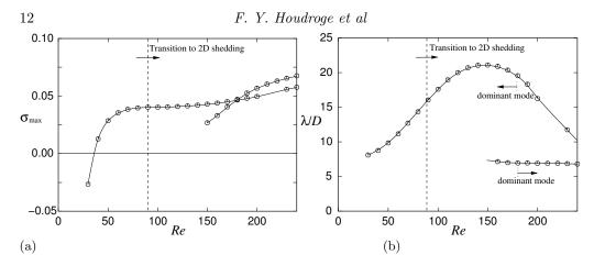
Figure 6: Left: (a) Maximum growth rate of the most unstable mode for transition from 2D steady to 3D steady flow. Right: (b) Variation of the wavelength of the fastest growing mode with the Reynolds number. Beyond  $Re \sim 150$  there are two peaks in the growth rate curve with the shorter wavelength peak developing the higher amplitude for  $Re \gtrsim 180$ .
