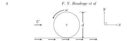
Figure 1: A two-dimensional schematic of the problem under consideration: a cylinder of diameter d is rolling along a wall. The translational and angular velocities are represented by U and  $\omega$ , respectively. In the simulations, the inertial frame of reference (x, y) is attached to the centre of the body.
