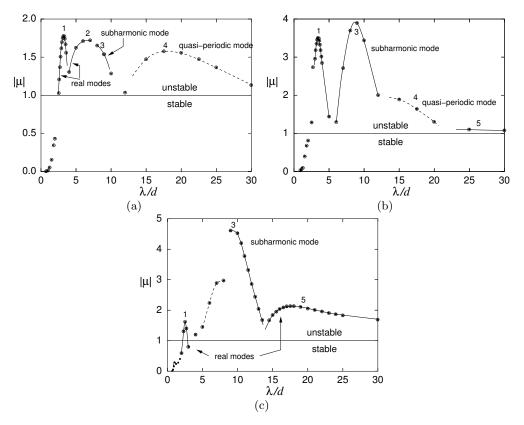
Figure 11: Floquet multiplier variation against spanwise wavelength for the dominant Floquet mode at each wavelength for Re = 100 (a), Re = 130 (b) and 160 (c).
