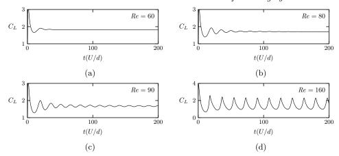
Figure 2: Time evolution (scaled by d/U) of the lift coefficient from impulsive startup. (a) & (b) Evolution for Reynolds number below the transition to 2D shedding. (c) & (d) Evolution for Reynolds numbers beyond the transition to vortex shedding.
