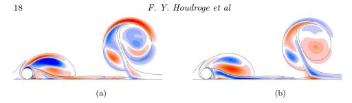
Figure 13: Visualisations of the streamwise perturbation vorticity for subharmonic mode (3) (left) and real mode (5) (right) at Re=160. These images depict streamwise perturbation vorticity coloured contours with base flow vorticity contour line at  $\pm 0.1 d/U$  overlaid to highlight the locations of the vortices.
