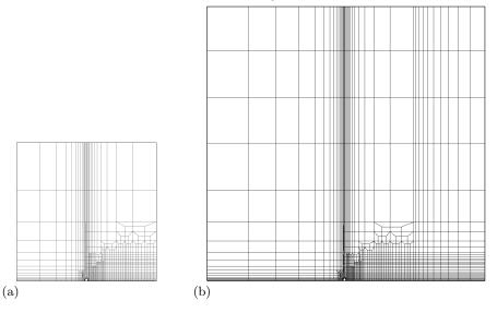
Figure 3: View of the cylinder mesh M1:  $(x_{1,u}, x_{1,d}, y_1) = (-25, 25, 50)$  (left image) and M2:  $(x_{2,u}, x_{2,d}, y_2) = (-50, 50, 100)$  (right image). The cylinder is placed in the middle of the x-axis, and near the wall at a gap ratio of G/d = 0.005 in order to avoid numerical singularities from arising. The flow is from left to right, and the resolution in the vicinity and downstream of the cylinder is increased in order to accurately capture the flow structures in the wake.
