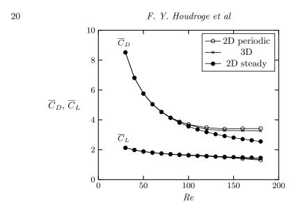
Figure 16: Comparison of time-averaged body force coefficients, drag  $\overline{C}_D$  and lift  $\overline{C}_L$ , between the two- and three-dimensional simulations for  $30 \leqslant Re \leqslant 180$ . Note that beyond  $Re_{c,2D}$  the 2D-steady predictions shown by the filled circles are based on flows calculated with the steady solver.
