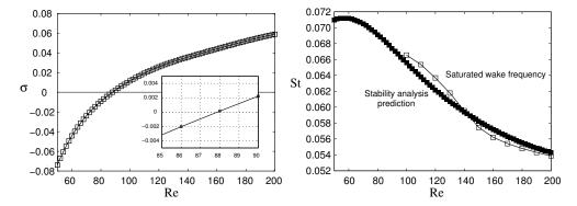
Figure 9: Left: Growth rate of most unstable mode from stability analysis applied to the rolling cylinder for  $50 \le Re \le 200$ . The lower inset shows the stability curve as it crosses the neutral stability line. Right: Predicted Strouhal number of the perturbation field compared to that of the saturated flow state.
