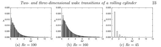
Figure 21: Time-mean amplitudes of saturated Fourier modes corresponding to the spanwise velocity component against dimensionless wavenumber kd for (a) Re = 100 and (b) Re = 160. These are taken over the 100 time units after the asymptotic state is reached. The righthand image (c) shows the final mode amplitude distribution for Re = 45, well below the transition to the periodic state.
