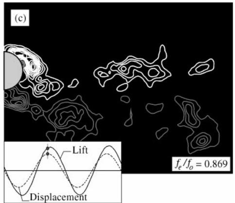
Figure 2. (a) Lift phase,  $\phi_{\text{lift}}$ , and amplitude of the lift coefficient  $C_L$  as a function of frequency ratio  $f_e/f_o$ , in which  $f_e$  is the excitation frequency and  $f_o$  is the Kármán frequency:  $\diamond$ , lift phase;  $\bullet$ ,  $C_L$ . Instantaneous vorticity fields are shown in (b) and (c). The time trace inserts show the instantaneous lift and displacement, where the timing of the image acquisition is indicated by a small circle.
