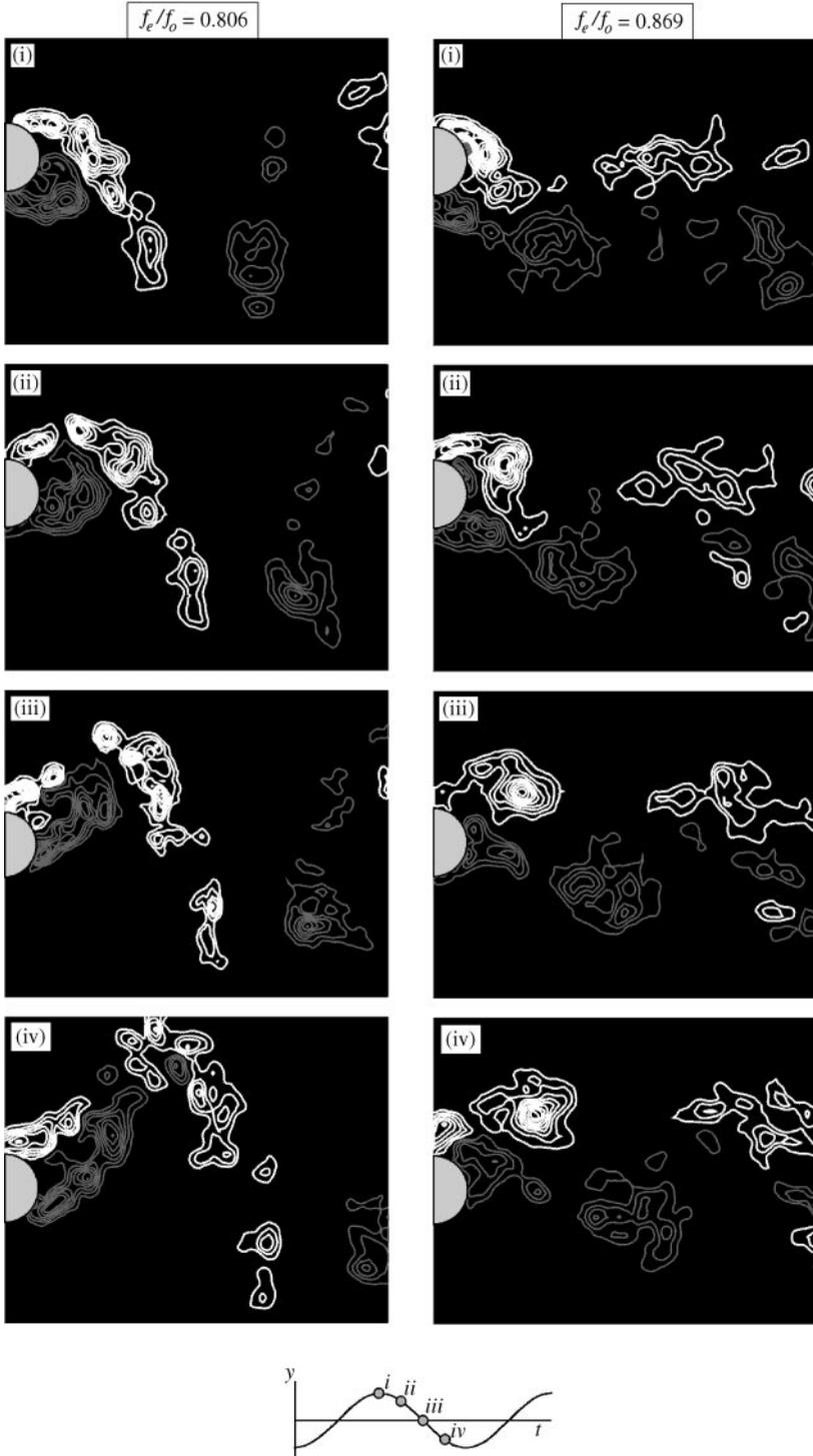
Figure 3. The evolution of vortex structures during the downward stroke of the cylinder. The left-hand side column shows the low-frequency wake mode before transition ( $f_e/f_o = 0.806$ ), while the high-frequency wake mode after transition ( $f_e/f_o = 0.869$ ) is on the right. The position of the cylinder for each image is shown in the displacement inserts beneath the fields.
