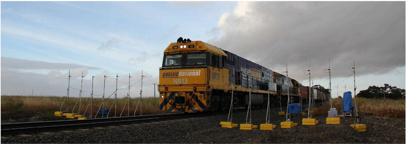
Fig. 1. An operational full-scale inter-modal freight train driving past measurement rakes of 4-hole dynamic pressure probes, placed either side of the train.
