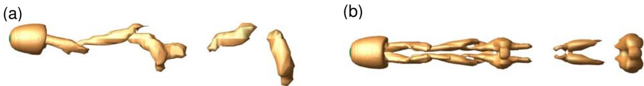
Fig. 4. Isosurface plots showing top (a) and side (b) views of the unsteady planar-symmetric wake computed at  $Re = 300$ , after rotation to its preferred orientation.
