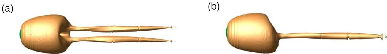
Fig. 2. The steady wake computed at  $Re = 250$ . Orthogonal top (a) and side (b) views are shown.
