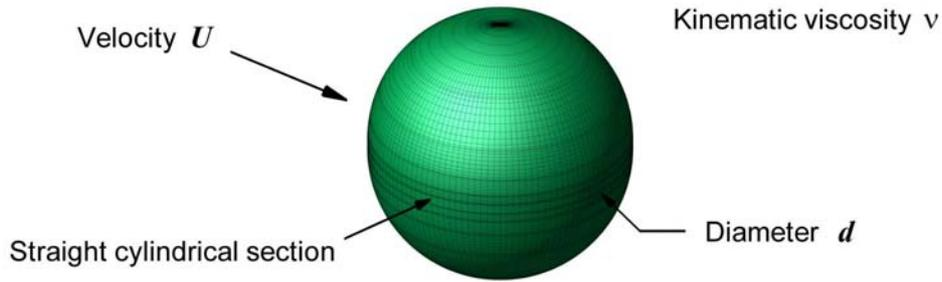
Fig. 1. The body used in the present study. The straight cylindrical section between the hemispherical ends has a length of  $0.04d$ , which gives it a volume and surface area 6% and 4% greater than a sphere with the same diameter.
