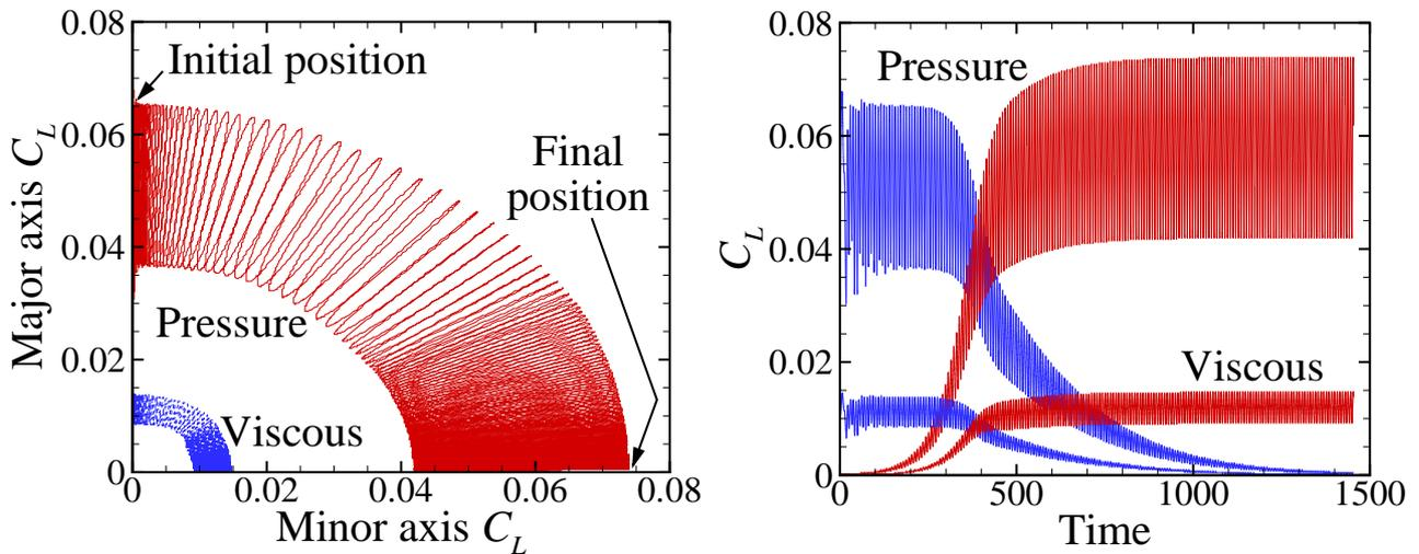
Fig. 3. Left: Phase plot of the viscous (dotted lines) and pressure (solid lines) lift coefficients acting on the spheroidal body at  $Re = 300$ . Initial and asymptotic orientations are labelled. Right: Time history of the lift coefficients measured in the major (blue) and minor (red) axis directions.
