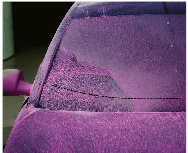
Fig. 30. View from the front of the model showing the flow over the end of the bonnet, windscreen and front of A-pillar. A dashed line is overlaid showing the positive bifurcation line of stagnation flow onto the rear windscreen.
