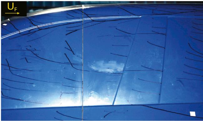
Fig. 32. View from the left side of the model of the A-pillars latter portion and side window, downstream of the mirror. Ink streaklines on the bottom edge of the A-pillar are observed to initially be transported along the roof beam's lower edge. ink droplets placed above the rear passenger window are associated with the A-pillar vortex structure being transported onto the roof, once the A-pillar vortex structure moves past the vehicle's B-pillar.
