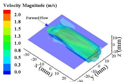
**Figure 3. Iso-surface plot of velocity magnitude downstream of the polymeric heart valve**
