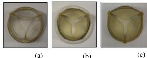
**Figure 1. The Three Prototype Designs of Polymeric Heart Valve; (a) Prototype A, (b) Prototype B, (c) Prototype C**
