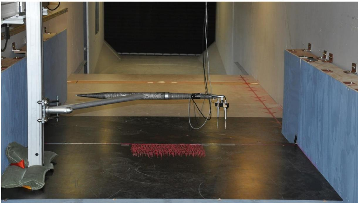
Figure 28: Two Cobra Probe configuration for two-dimensional traversing. Traversing vertically and in the stream-wise direction. Note the weight bags for vibration damping at the base of the vertical traverse on the left.
