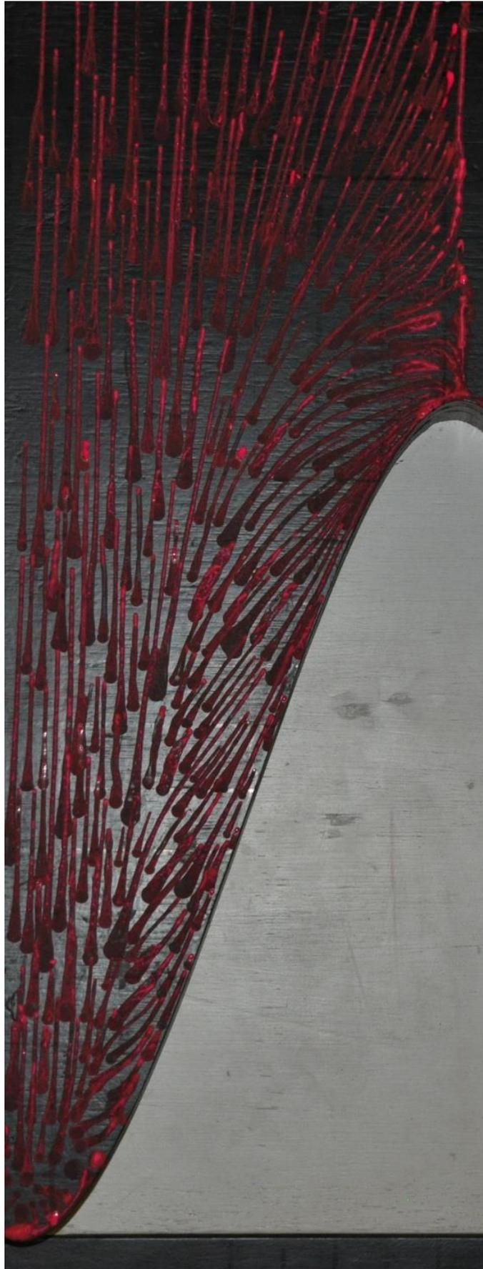
Figure 139: Surface shear stress visualisation over Sinusoidal FFS:  $A/\lambda = 1$ .
