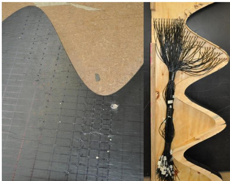
Figure 39: Surface of pressure tapped sinusoidal model (Left). Underside of pressure tapped model, showing 1 m long tubes (Right).
