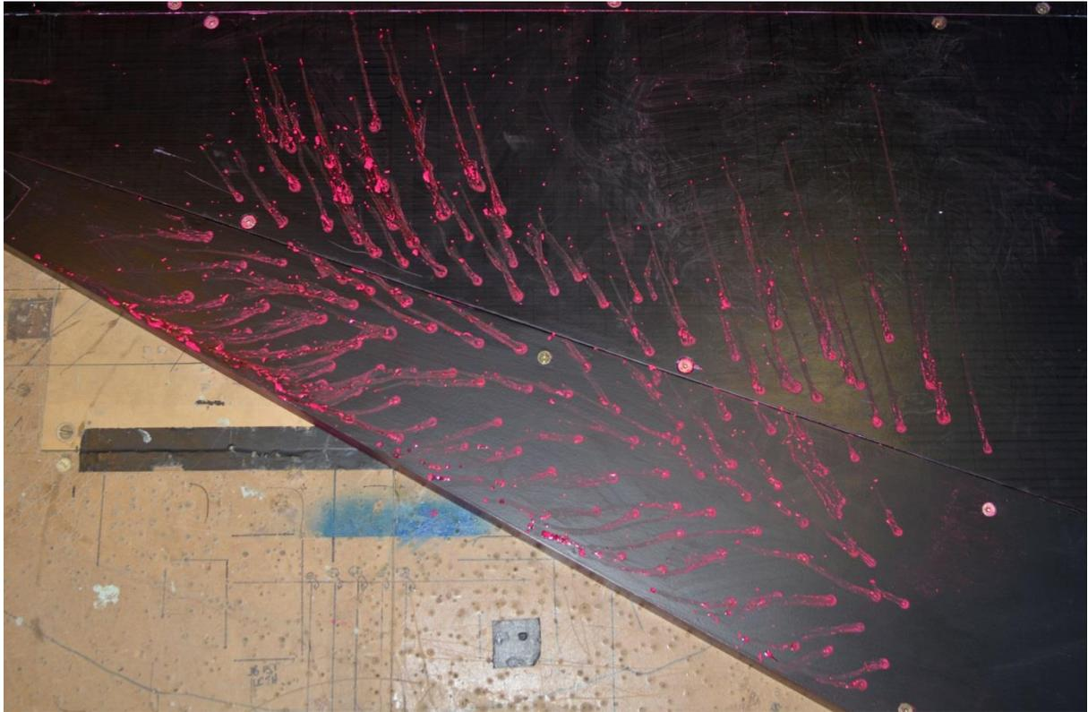
Figure 168: Paint droplet surface shear stress visualisation for  $\delta/h = 2.7$ . Yaw angle,  $\theta = 30^\circ$ . Inflow Configuration 1. Step height,  $h = 50$  mm. Flow direction from bottom of page to top.
