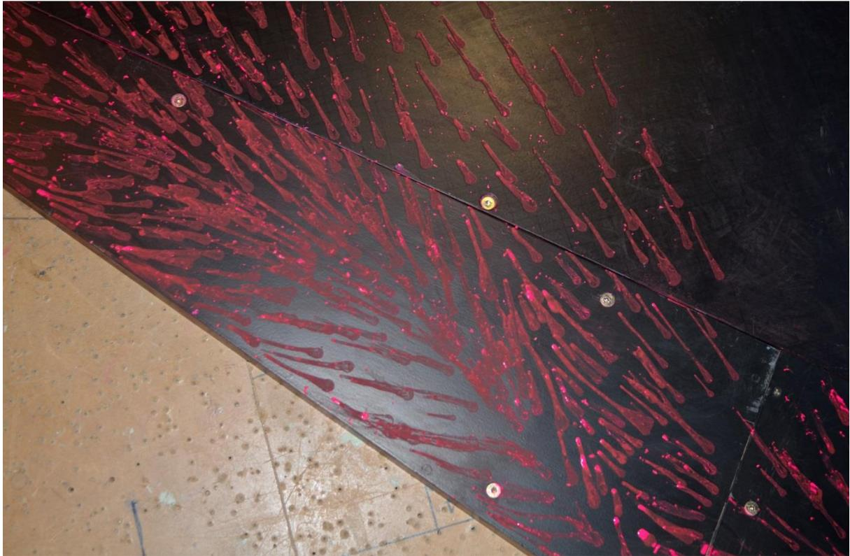
Figure 172: Paint droplet surface shear stress visualisation for  $\delta/h = 2.7$ . Yaw angle,  $\theta = 50^\circ$ . Inflow Configuration 1. Step height,  $h = 50$  mm. Flow direction from bottom of page to top.
