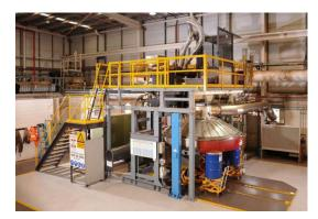
**Figure 1**: The semi-industrial scale (3 m in diameter) integrated dry granulation and heat recovery pilot plant at CSIRO.
