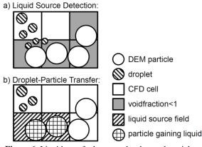
Figure 6: Liquid transfer between droplets and particles, via Eulerian liquid source field.
