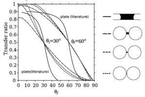
Figure 4: Liquid-bridge transfer ratios depending on the contact angle  $\Theta$  (left). Differing bridge configurations are shown schematically (at right) with varying line/dash types for two plates; particles with V=0.001; particles with V=0.0001 and particles with V=0.00001., Shi and McCarthy (2008).
