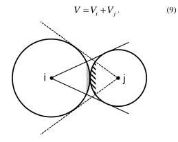
**Figure 3**: Schematic sketch of spherical cap denoting the liquid contributing to the formation of a liquid bridge.
