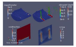
**Figure 8**: Droplet-particle liquid transfer rate (upper left), droplets and liquid carried on particle surface (upper right), voidfraction field (lower left) and gas velocity (lower right).
