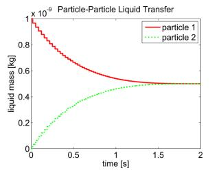
**Figure 5**: Liquid transfer between a (initially) dry and wet particle bouncing on each other. Both particles have the same liquid contact angle.
