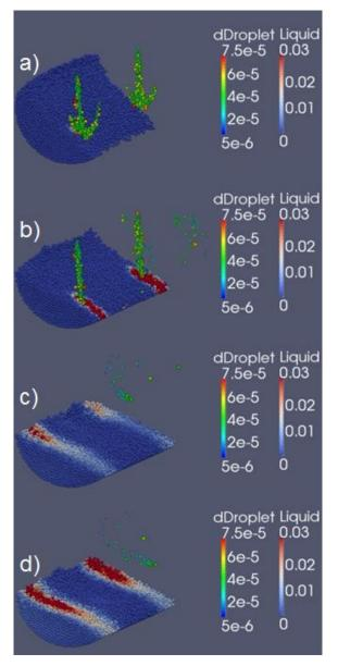
**Figure 7**: Liquid transfer from droplets to particles as well as particle-particle liquid transfer for a) t=0.35s, b) t=3.5s, c) t=5.75s, e) t=11 s.
