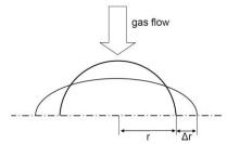
Figure 2 Axisymmetric representation of an oscillating, distorted droplet.
