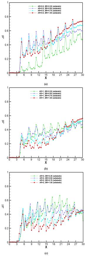
Figure 6: Predicted laterally averaged  $\eta$  distribution on the lining wall along the stream-wise direction under different blowing ratios; (a) AR=0.5, (b) AR=1, (c) AR=2.
