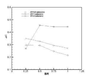
**Figure 7:** Relationship between area-averaged η values and blowing ratios for three tested elliptic hole's aspect ratios (adiabatic heat transfer model).
