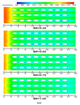
Figure 8: Predicted wall temperature distributions on lining wall under different blowing ratios with conjugate heat transfer model: (a) AR=0.5, (b) AR=1, (c) AR=2
