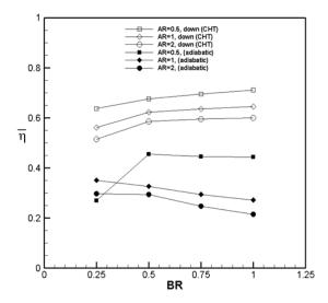
Figure 9: Relationship between area-averaged  $\eta$  values and blowing ratios for three tested elliptic holes (conjugate heat transfer model).
