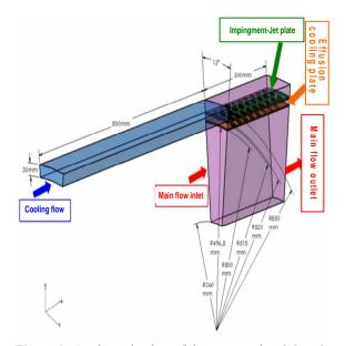
Figure 1: A schematic view of the computational domain for effusion cooling lining wall in a circular combustion chamber.
