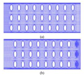
Figure 2: Surface grid distribution for elliptic hole with aspect ratio (AR) of 0.5 on ; (a) impingement jet hole plate; (b) lining wall.
