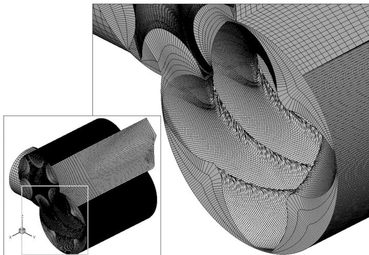
Fig. 3. The 3D grid used for the flow calculation.
