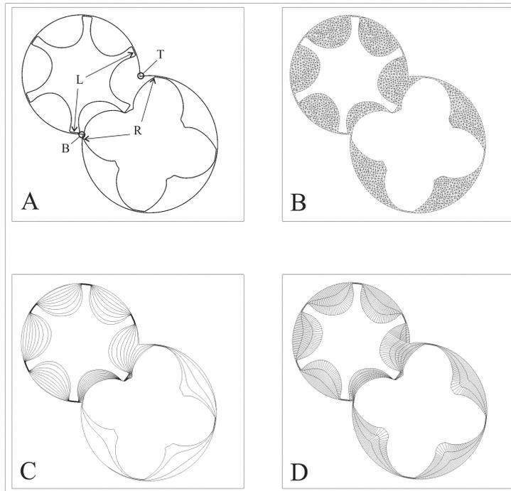
Fig. 1. Three steps in the generation of structured grids: (a) domain; (b) unstructured grid; (c) potential solution obtained on the unstructured grid; (d) final structured grid based on the potential solution.
