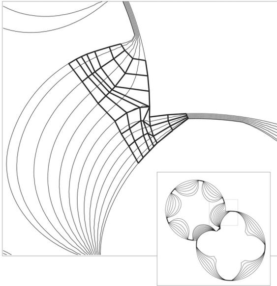
Fig. 2. Poor quality grid around CUSP T due to constant potential boundary condition.
