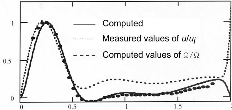
Fig. 1. Comparison of angular velocity and axial velocity component along the axis for  $Re = 1560$ . Data were provided by Okulov et al. [7].
