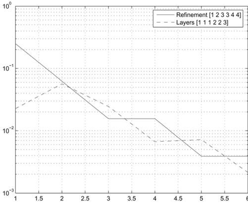
Fig. 3. The error indicators during six iterations in the adaptive algorithm.
