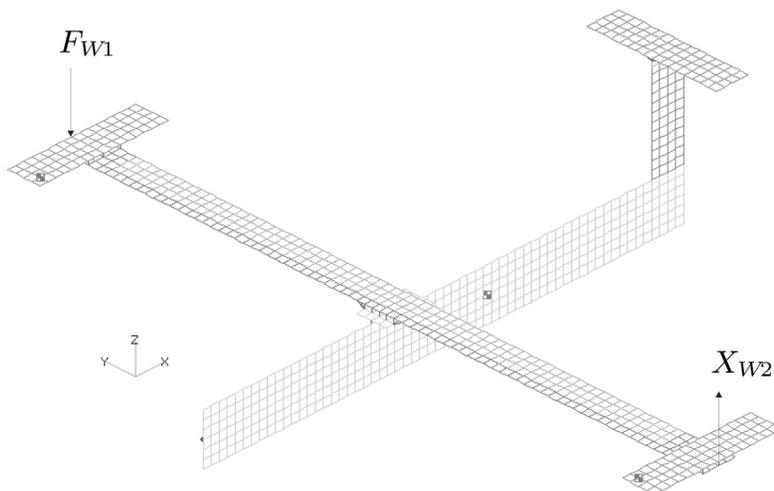
Fig. 2. Finite element model of the Garteur aircraft.
