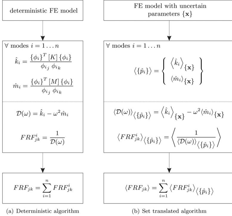
Fig. 1. Translation of the deterministic modal superposition algorithm to an equivalent IFE procedure.
