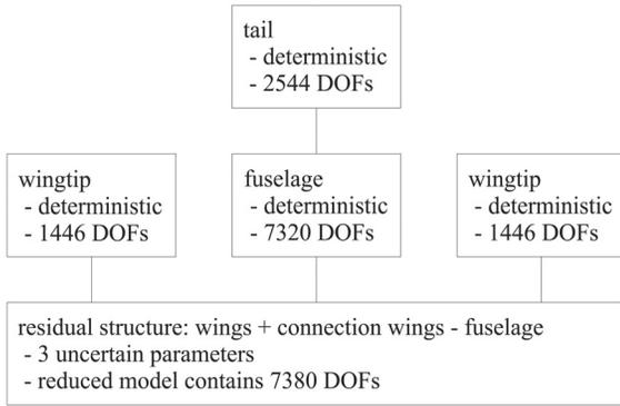
Fig. 3. Overview of the substructured Garter aircraft.
