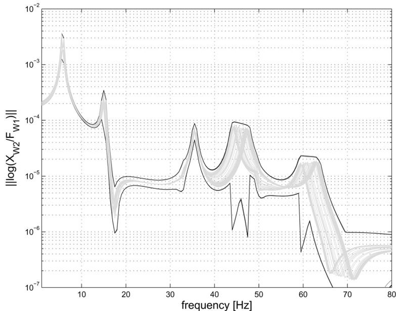
Fig. 4. Amplitude of the damped interval FRF of the Garter aircraft model, compared with 100 Monte Carlo samples.
