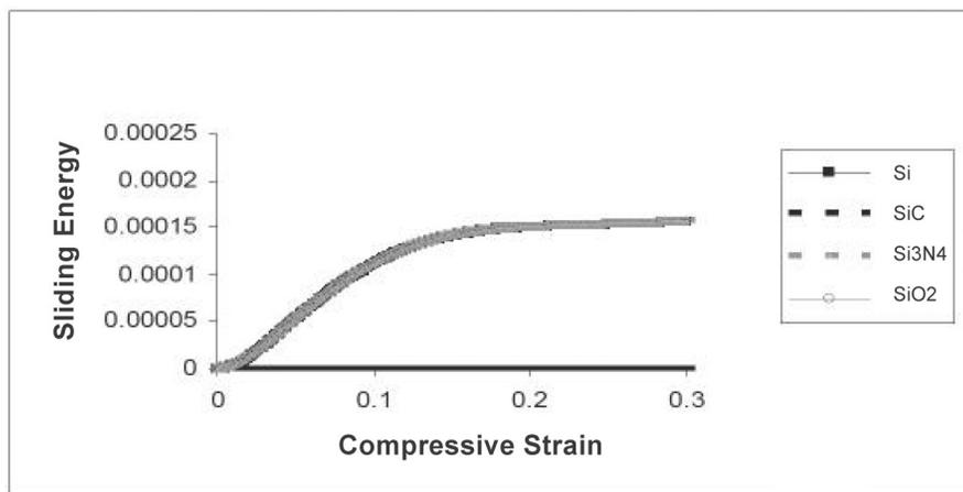
Fig. 3. Compressive strain vs energy dissipated due to the sliding.
