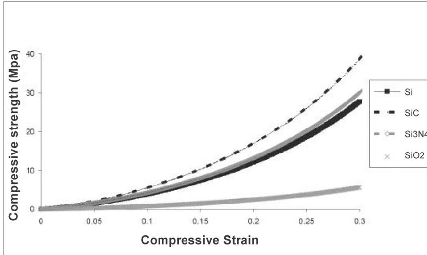
Fig. 1. Compressive strain vs compressive strength.
