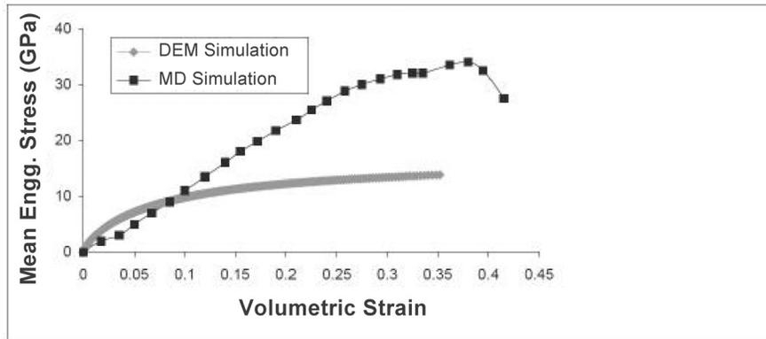
Fig. 4. Mean strength of Si assembly during tri-axial compression.
