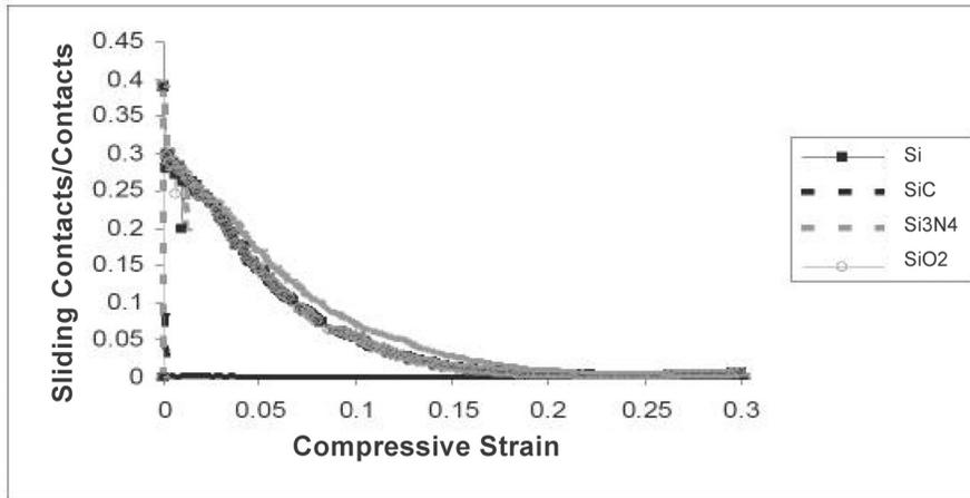
Fig. 2. Compressive strain vs proportion of sliding contacts.
