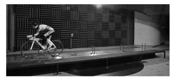
**Figure 2.3.5** - Multi-Rider Cycling Rig shown with mannequin mounted at Position 1. Struts are visible for each of the four force balances that mount at the bicycle rear wheel.
