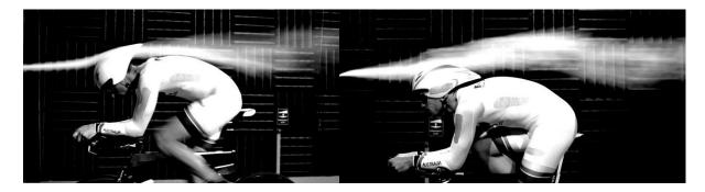
**Figure 5.1.4** - Left; flow over lead cyclist in tandem pair. Right; flow over trailing cyclist with bicycle length separation between riders
