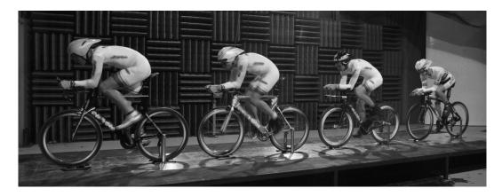
**Figure 2.7.7** - Team formation on rig in wind tunnel test section (displaying Sequence 1 in descending size order)
