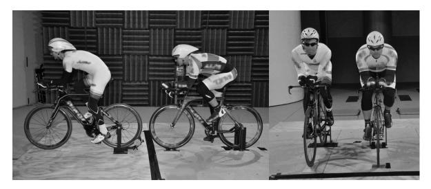
**Figure 2.7.3** – (Left) Riders in tandem formation with instrumented rider trailing; (Right) Riders in side-by-side (transverse) formation with instrumented rider on right of image.
