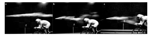
**Figure 5.1.5** - Flow profile ahead of the trailing cyclist at a bicycle length downstream of the lead rider. Three injection points shown, indicated by wand location, highlighting the difference in flow profile with vertical height
