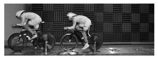
Figure 2.7.9 - Athletes mounted on Multi-Rider Cycling Rig at minimum separation
