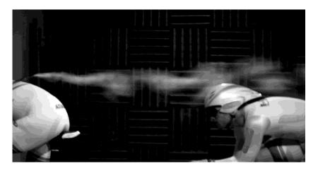
**Figure 5.1.2** - Smoke injected immediately upstream of separation point on the lead cyclist. Riders positioned at minimum separation. Both athletes pedalling during test.
