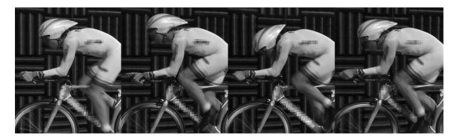
Figure 2.7.8 - Body positions used during testing; (L-R) baseline, head raised, head lowered, elbows together
