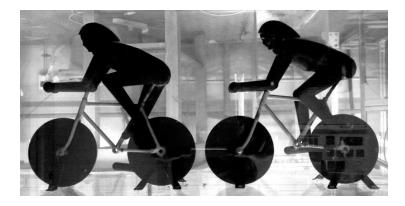
**Figure 2.7.10** – Cyclist models mounted on ground plane and suspended in the water channel. Shown at minimum separation distance (Spacing 1).
