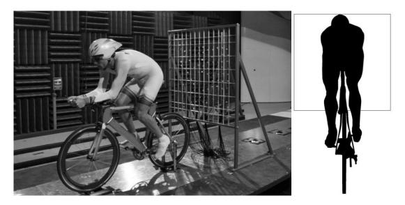
**Figure 2.7.17** – (L) Single rider setup with pressure grid 600mm downstream of athlete. (R) Depiction of the interrogation window in the cyclist wake.
