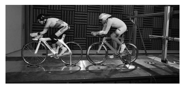
**Figure 2.7.14** - Tandem setup in wind tunnel depicting mannequin and athlete with traverse and probe arrangement downstream of the athlete
