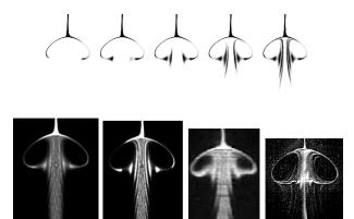
The flow field was found numerically for a Reynolds number of 1850 and an aspect h/D = 1.75. A recirculation bubble is found on the central axis, similar in general shape to that observed experimentally except that it has a closed form and is constrained to be purely axisymmetric. To the left, top row, is shown successive stages of tracer particles approaching the lower stagnation point of the bubble. The generation of the density variation predicted analytically is clearly seen.
