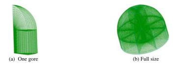
Fig. 2. The hemispherical parachute calculation grid.
