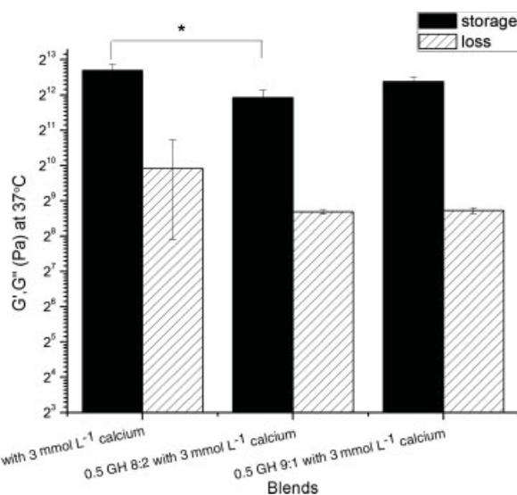
**Figure 2.** Storage  $G'$  and loss  $G''$  moduli of gellan and gellan/HPMC of various ratios at 37 °C. Comparison of storage and loss moduli obtained at 10 Hz (\*significant difference at  $p < 0.05$ ,  $n = 3$ ).
