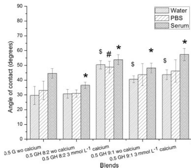
**Figure 4.** Contact angle measurements with water, PBS and serum of gellan/HPMC gels (with and without (wo) the addition of calcium). \*, Significant difference of serum contact angle as compared to 0.5% gellan without calcium at  $p < 0.05$ ; #, significant difference of PBS contact angle as compared to 0.5% gellan without calcium at  $p < 0.05$ ; \$, significant difference of water contact angle as compared to 0.5% gellan without calcium at  $p < 0.05$ .
