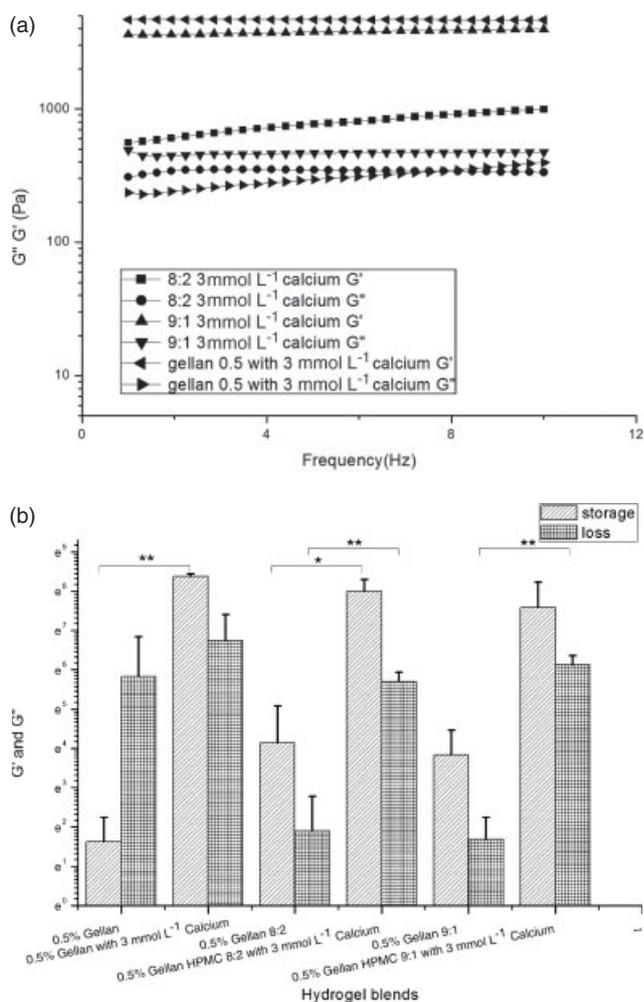
**Figure 1.** Storage  $G'$  and loss  $G''$  moduli of gellan and gellan/HPMC of various ratios. (a) Frequency sweep of gellan and gellan/HPMC blends from 1 to 10 Hz. (b) Comparison of storage and loss moduli obtained at 10 Hz (\*significant difference at  $p < 0.05$ ,  $n = 3$ ; \*\*significant difference at  $p < 0.005$ ,  $n = 3$ ).
