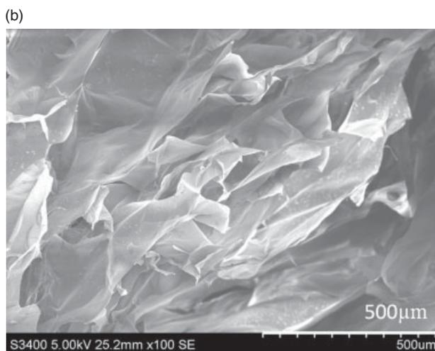
**Figure 5.** SEM micrographs of gellan/HPMC gels: (a) 0.5GH8:2 with 3 mmol L<sup>-1</sup> calcium; (b) 0.5GH9:1 with 3 mmol L<sup>-1</sup> calcium.
