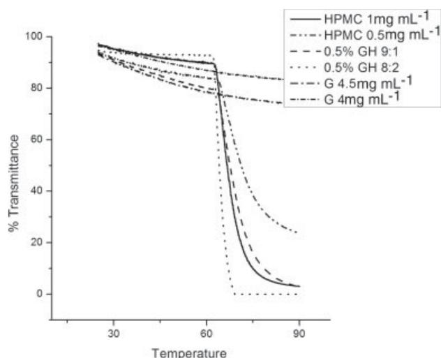
**Figure 3.** Cloud point plots for various ratios of gellan and HPMC (as indicated) without the addition of calcium, with a temperature sweep from 25 to 90 °C.
