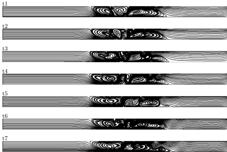
Fig. 21. (a) Variations of Nu_F with time at Ra = 2 \times 10^7 and Pe = 40 , and (b) streamlines of flow behaviour at different times indicated in (a).
