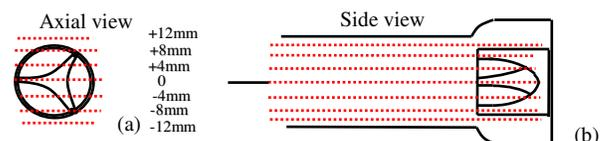
Figure 2. Location of measurement planes (dotted lines)
